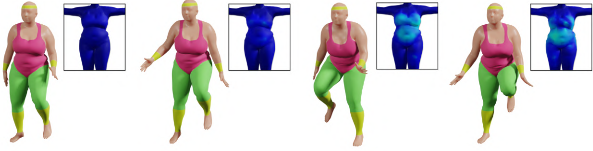
Figure 9: Our model incorporates skeletal tracking of target input animations through control forces. Note that even in the absence of external interactions, dynamic deformations appear as an effect of inertial components. The figure shows a sequence of three animation frames and a colormap with the corresponding vertex displacements in unposed space (insets).
