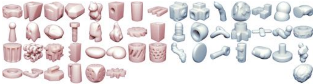
Figure 8: Collider objects (all from Thingi10K [Zhou and Jacobson 2016]) used for training (left, in red) and quantitative testing (right, in blue) our deformation model. Average error of our model is 17.0% on the train colliders and 17.8% on the test colliders, demonstrating its generalization capabilities.
